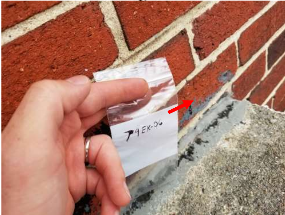
Photograph #0003 Tar-and-gravel portion – Historical grey roof sealant (5% Chrysotile)
