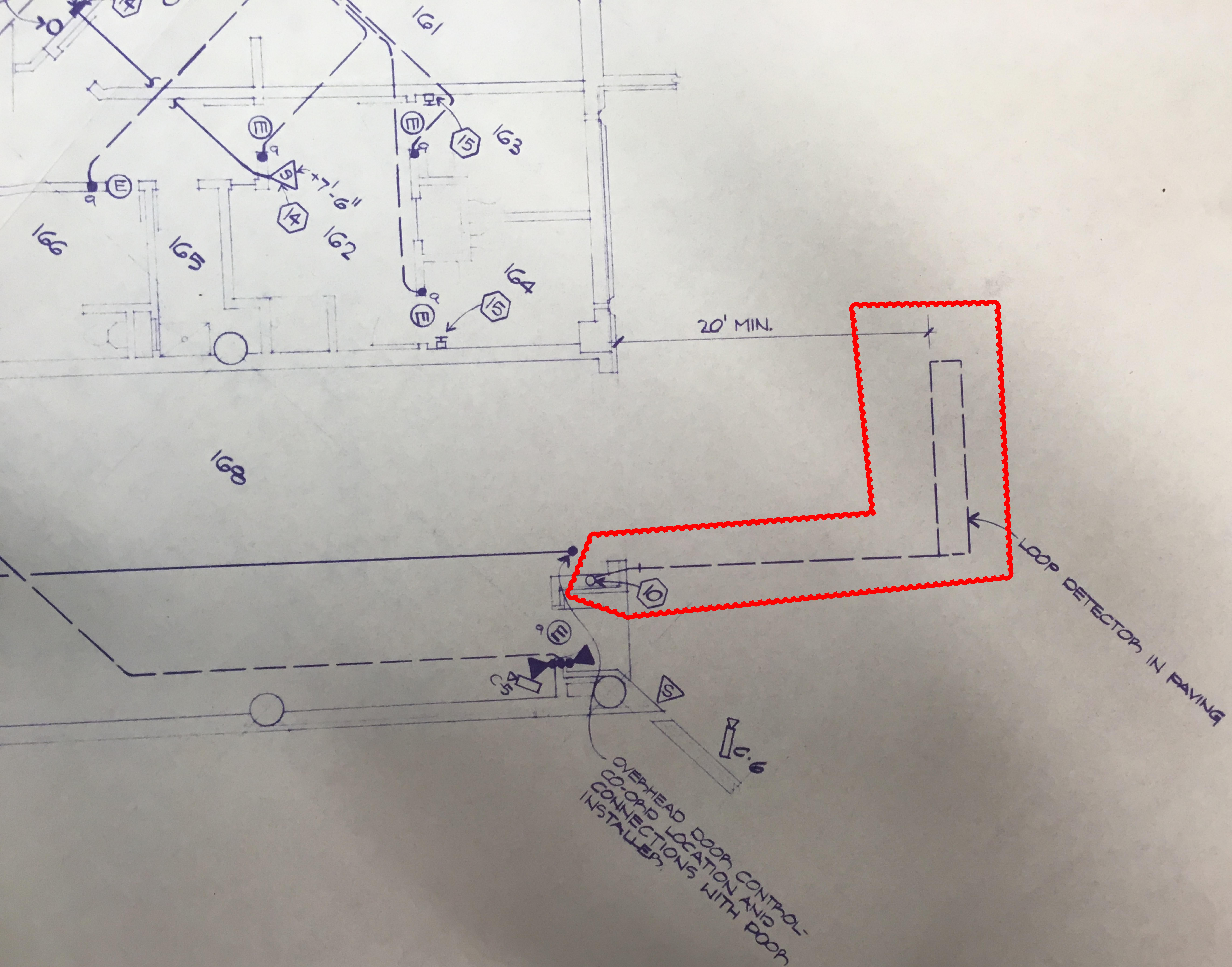
STUB ALL CONDUITS, ENTERING AREA FROM FLOOR, UP 6" ABOVE CONCRETE. ALL CONDUITS ENTERING FLOOR SPACE FROM ABOVE SHALL BE TERMINATED 3" BELOW REMOVABLE FLOOR. ALL CONDUITS TERMINATED IN THIS AREA SHALL HAVE BUSHINGS INSTALLED.
