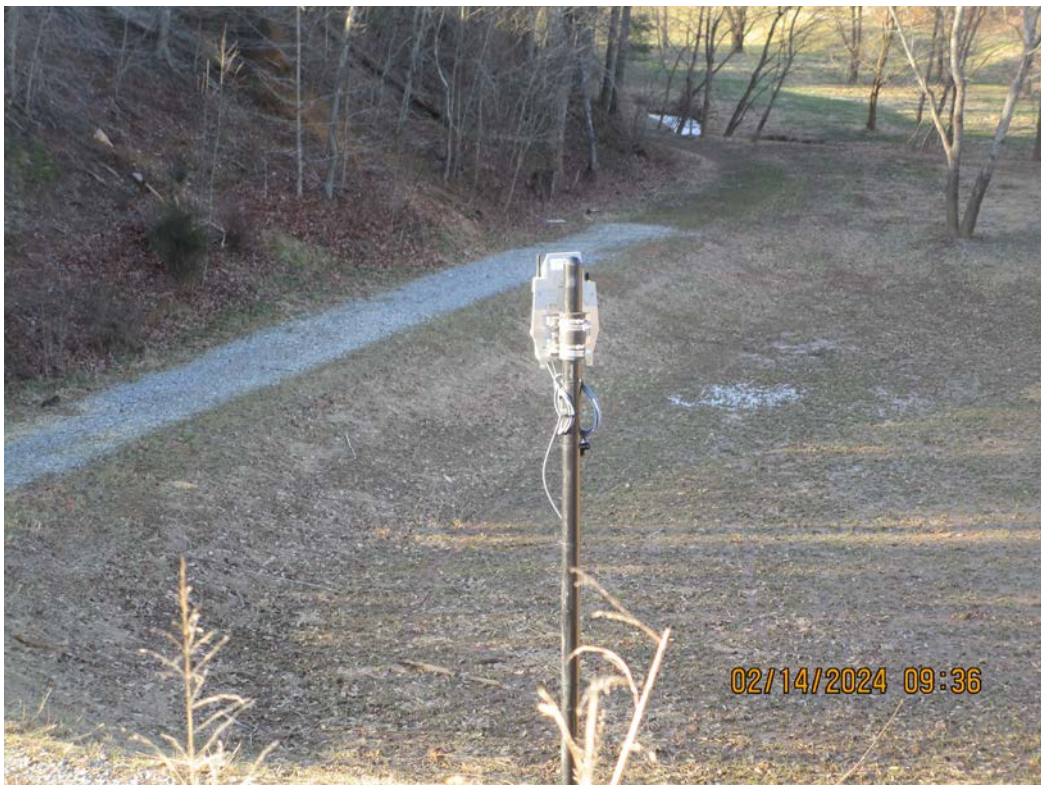
High Water Monitor with Cell Communications and Solar Power
