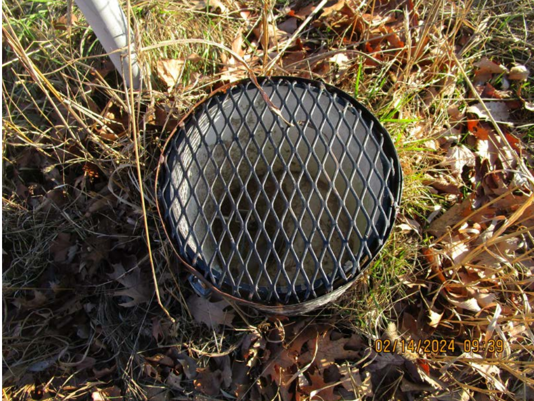
Stillwell w/ Pressure Transducer for High-Water Monitoring/Alert System
